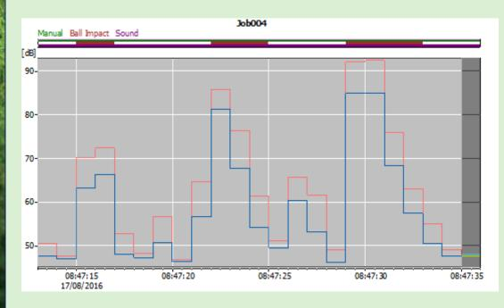
$L_{Aeq,1s}$  (blue) and  $L_{AFmax,1s}$ (red) levels recorded during three instances of a football impacting the perimeter fence of the pitch when kicked from a distance of 10 m.  $L_{Aeq,1s}$  levels; 63, 81 and 85 dB respectively with corresponding  $L_{AFmax}$  levels; 70, 86 and 92 dB.
