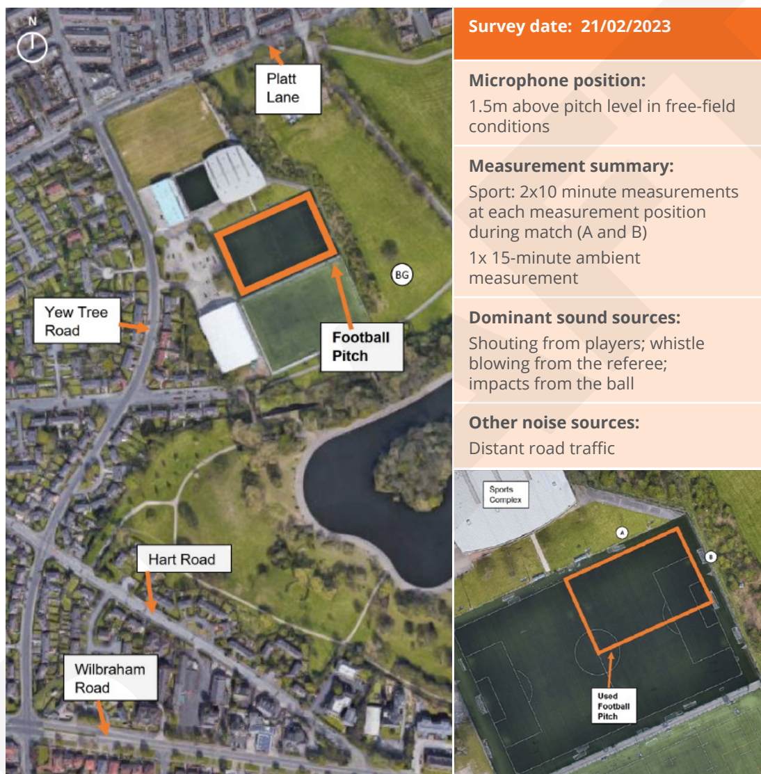
Figure 13.4 / Figure 13.5: Site layout and monitoring locations
