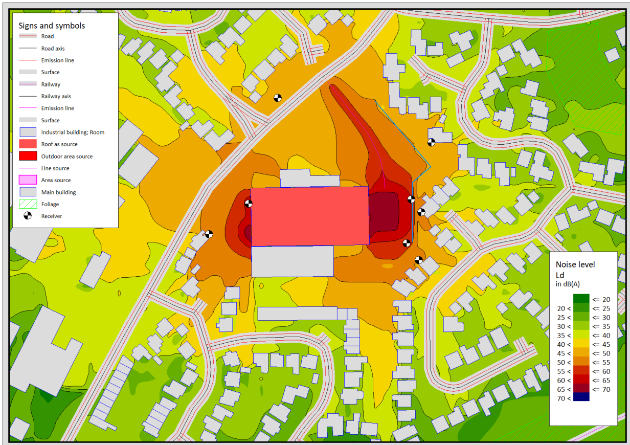
Figure 4 – Soundplan model for noise barrier and fencing only
