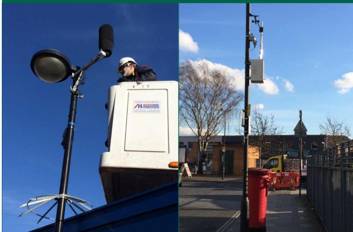
Figure 12: Example of sound level meter installations on lamp-posts
