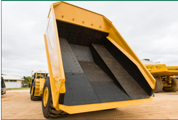
Figure 6: Rubber lined payload areas on dumper trucks
